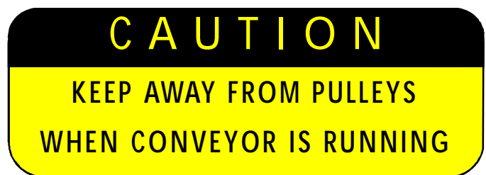
ABOVE: Label placed near all pulleys (center drives, end drives, tail pulleys)
