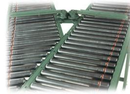
Traffic cops control merges allowing first carton striking an arm to pass. This action automatically locks the other arm in place until the first carton clears the arm. Model TC shown attached to optional conveyor.
